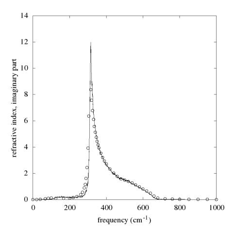
Figure 2: Imaginary part of the refractive index versus frequency for a LiF crystal at 300 K. As in figure 1, circles are experimental data taken from [1], while solid line is obtained, through Green–Kubo theory, from MD simulations for the motions of a system of 4096 ions.
