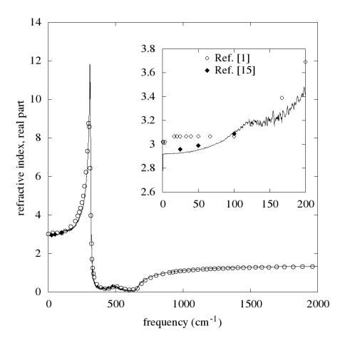
Figure 1: Real part of the refractive index versus frequency for a LiF crystal at 300 K. Circles and diamonds are experimental data taken from [1] and [15] respectively. Solid line is obtained, through Green–Kubo theory, from MD simulations for the motions of a system of 4096 ions. The inset is a zoom of the leftmost part of the figure.
