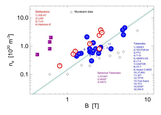
FIG. 1. Density limit values vs B for various machines: conventional tokamaks, for which recent data are shown (see references 32–47) along with the original ones of Murakami (see 31), stellarator machines  $^{48-51}$ , and spherical tokamaks  $^{52-54}$ . Dotted line is the theoretical density limit (11).
